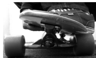
HEEL-SIDE WHEEL BITE CHECK
