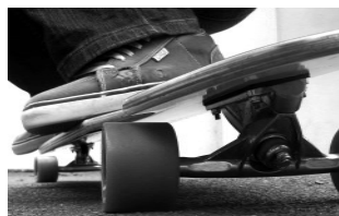
TOE-SIDE WHEEL BITE CHECK
